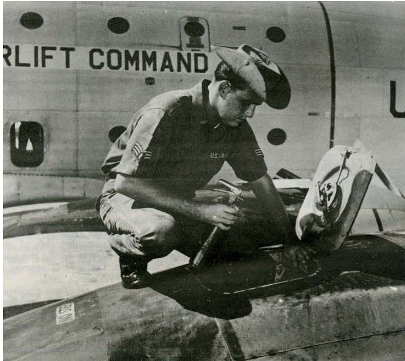
A C-124 was saved here recently from fire by A1C Garland B. Miller Jr., shown here demonstrating how he went back into the nacelle of the burning craft to extinguish the flames. Miller was checking out an auxiliary unit in the nacelle when the asbestos wrapping on the exhaust pipe began smoking and burst into flames. The aircraft saved by the airman belongs to the 63rd Military Airlift Wg. at Hunter AFB, Ga.
